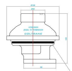
coltrane, B-Klep, RC-T-B, Pnom 25mbar, Pb 15mbar, Q-max 6 m3st/h lucht - 7,5 m3/h aardgas, Batch DD/MM/YY GastecQA 🗅
