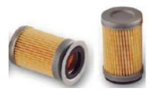
Filter cartridge consisting of an inner spring made of galvanised steel supporting an outer structure of pleated filter paper and two zinc-plated steel covers glued with a petroleum derivative resistant adhesive.
